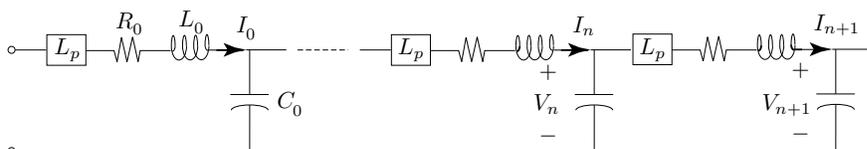
Figure 2.4.5 Transmission line loaded with Pupin coils.
