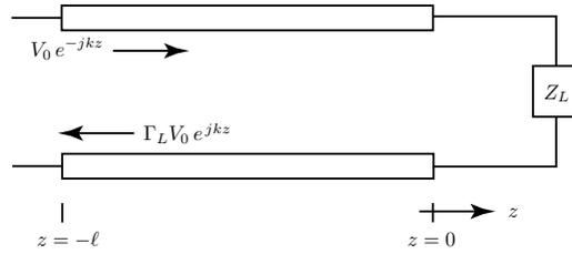
Figure 2.3.1 Transmission line with termination  $Z_L$ .
