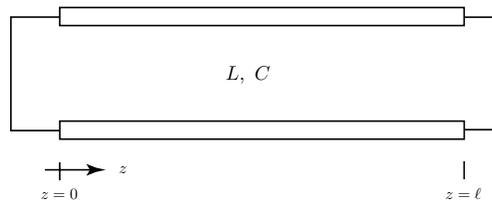
**Figure 2.2.7** Transmission line with  $V(z = 0) = 0$  and  $I(z = \ell) = 0$ .
