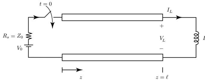
Figure E2.2.3.1 Transmission line with inductive termination.
