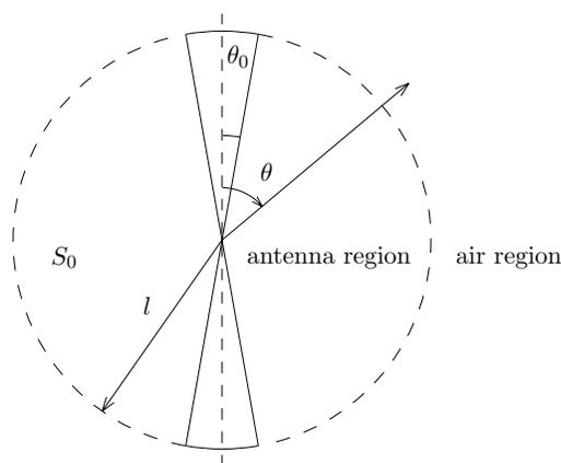
Figure 5.6.1 Biconical antenna.
