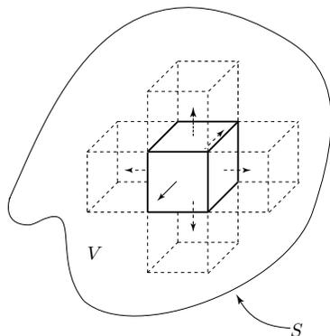
**Figure 1.1.3** Derivation of divergence theorem.
