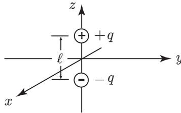
Figure 1.4.1 Hertzian dipole.
