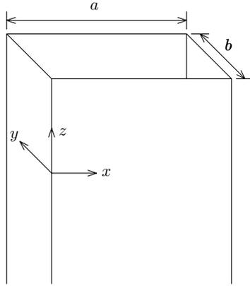
Figure 4.2.17 Metallic rectangular waveguides.
