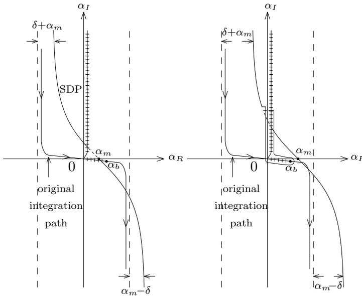
Figure 5.7.13 (a) The SDP is to the left of the branch point and the saddle point  $\alpha_m$  occurs on the lower Riemann sheet where  $k_{zI} < 0$ . (b) The SDP is to the right of the branch point and the saddle point  $\alpha_m$  occurs on the top Riemann sheet where  $k_{zI} > 0$ .
