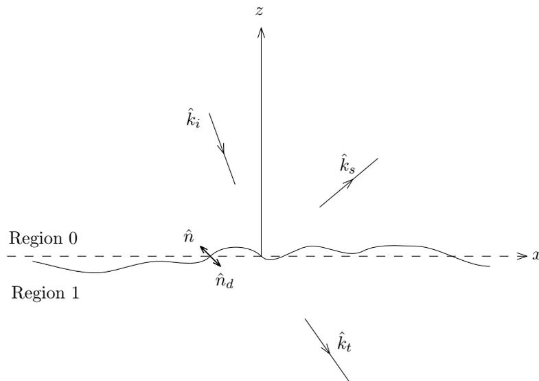
Figure 7.4.1 Scattering by a random rough surface.
