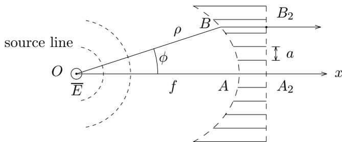
Figure 6.4.9 Metal-plate lens.
