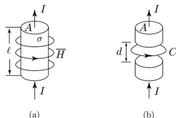
Figure 2.1.6 Displacement current.
