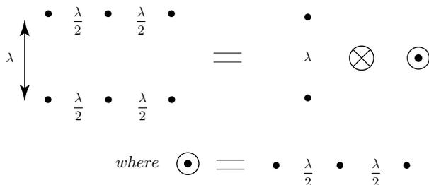
Figure E2.5.5.1 Six-dipole two-dimensional array.
