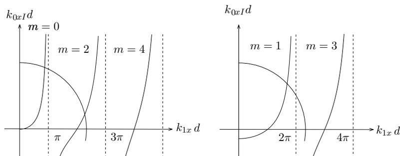
Figure 4.2.15 Graphical determination of  $k_x d$ .
