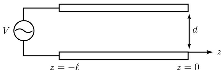
Figure E2.2.1.1 Open-circuited transmission line as capacitor.
