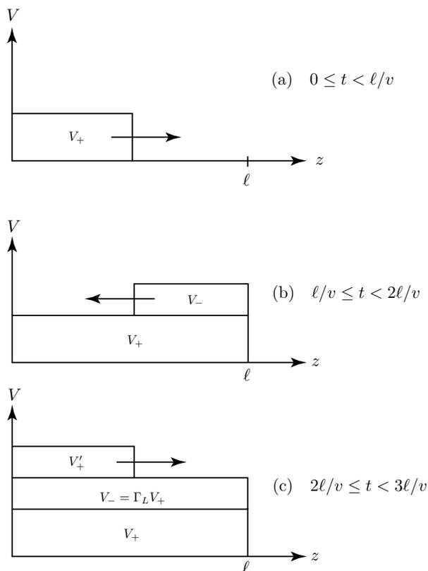
**Figure 2.2.3** Transient build-up on a transmission line.
