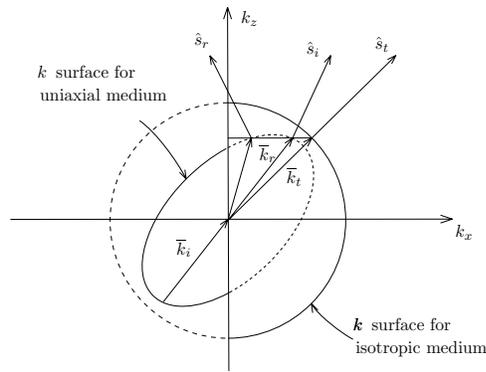
Figure 4.1.10 Wave vector directions and power flow directions.
