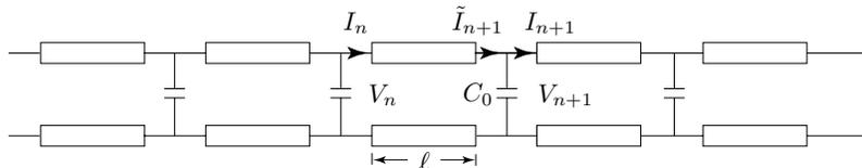
Figure E2.4.3.1 Periodically loaded transmission line.
