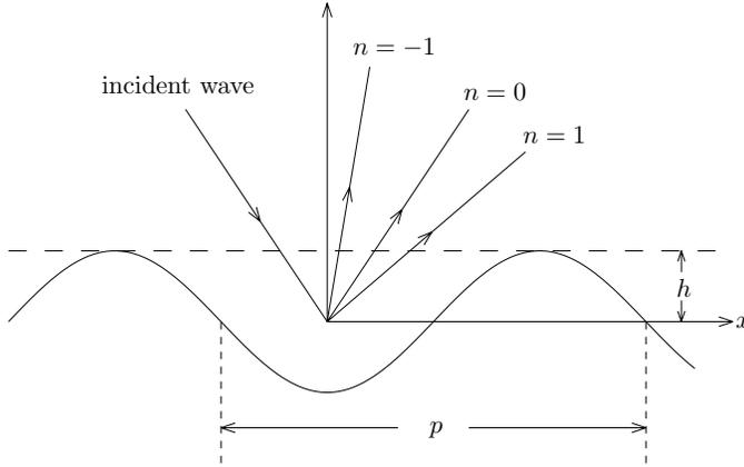
Figure 7.3.2 Scattering by a periodic rough surface.
