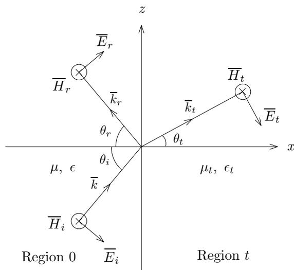
Figure 4.1.1 Reflection and transmission of TM waves.
