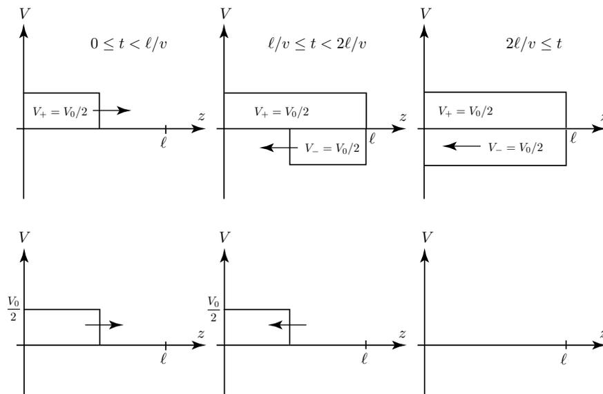
Figure 2.2.5 Transients on a shorted circuit line.
