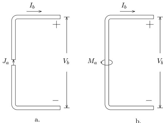
**Figure E6.2.2.1** a. Reaction of a current source. b. Reaction of a voltage source.
