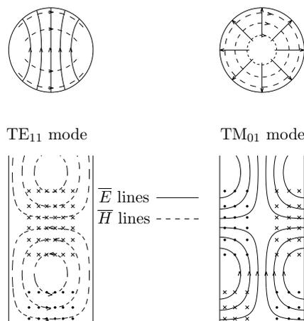
Figure 4.2.25 Field lines for  $\text{TE}_{11}$  and  $\text{TM}_{01}$  modes.
