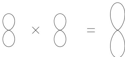
Figure E2.5.6.1 Multiplication of two two-dipole array patterns.
