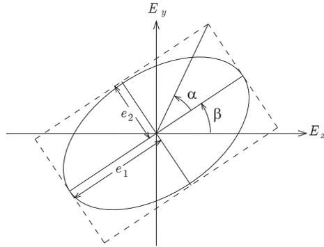
Figure 1.2.10 Elliptical polarization.
