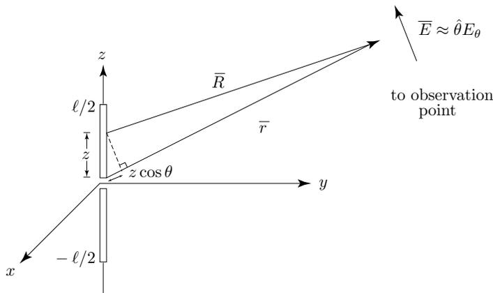
Figure 2.5.4 Calculation of radiation electric field by superposition.
