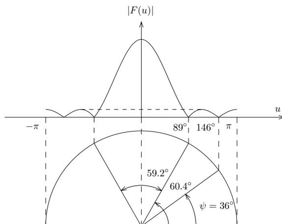
Figure E5.4.7.2 Array factor for Case 3.
