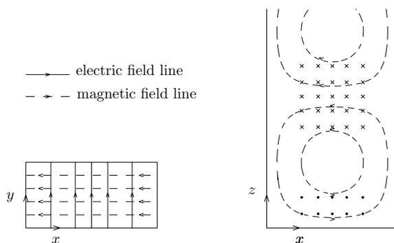
Figure 4.2.19  $\text{TE}_{10}$  mode in a rectangular waveguide.
