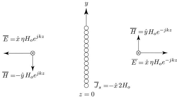
**Figure 2.5.10** Current sheet for the reflected wave.
