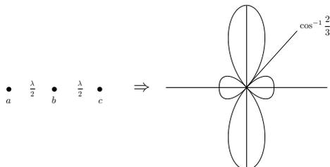
**Figure E2.5.3.4** Radiation pattern of three dipoles in phase.
