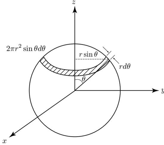
Figure 1.4.4 Integration geometry for time-average power density.
