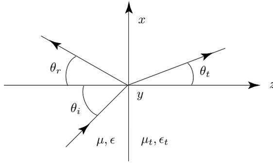
Figure 2.5.1 Reflection and transmission at a plane boundary.
