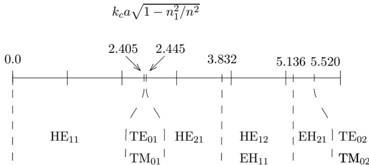
**Figure 4.2.27** Cutoff of circular dielectric waveguide modes.
