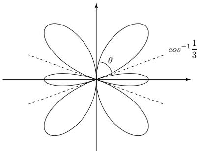
Figure 2.5.6 Radiation pattern for  $3\lambda/2$  linear antenna.
