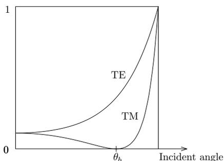
Figure 1.7.6 Reflectivity of TE and TM waves.
