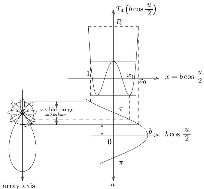
Figure 5.4.7 Endfire Dolph-Chebyshev array with  $N = 5$  and  $kd = \pi/2$ .
