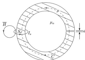
**Figure 2.1.8** Magnetic circuit excited by current loop.
