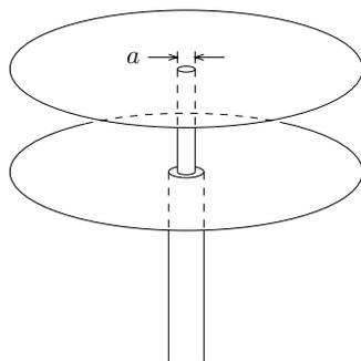
Figure 6.2A.2 Probe excitation of a radial parallel-plate waveguide.
