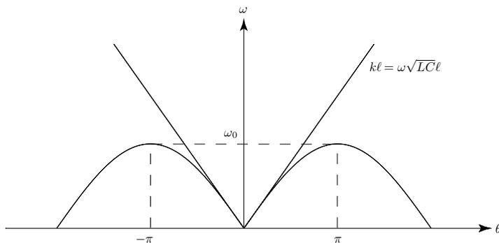
Figure 2.4.3 Dispersion relation for low-pass transmission line.
