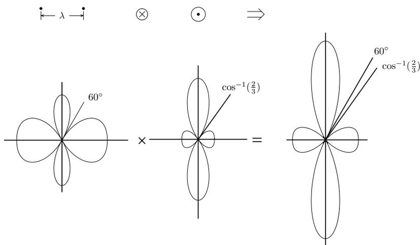
Figure E2.5.4.2 Radiation pattern of five-dipole array.
