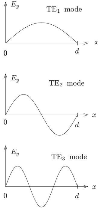
**Figure 4.2.5** Field amplitudes for TE<sub>1</sub>, TE<sub>2</sub>, and TE<sub>3</sub> modes.
