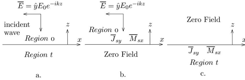
**Figure E6.1.1.1 Extinction Theorem a. Plane wave incident upon a boundary surface. b. Incident wave and equivalent electric and magnetic current sheets placed in Region 0. c. Equivalent electric and magnetic current sheets placed in Region t.**
