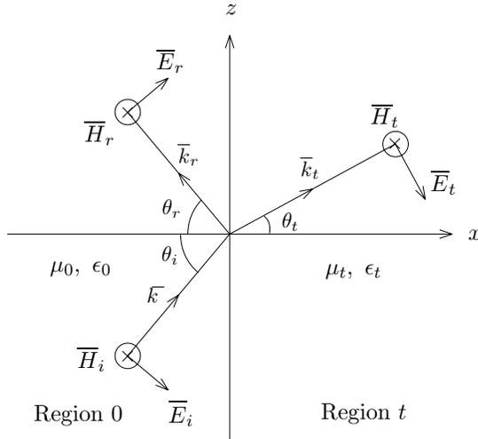
Figure 1.7.4 Reflection and transmission of TM waves.
