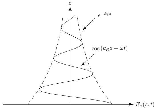
Figure 3.1.2 Wave in dissipative medium at  $t = 0$ .
