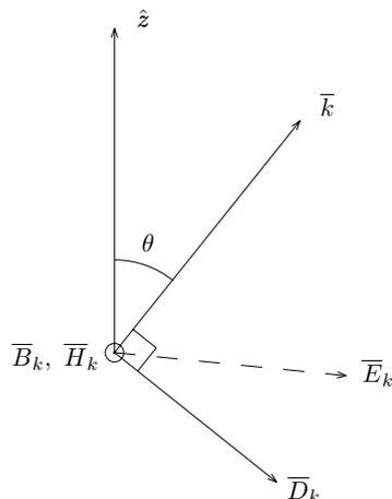
Figure 3.3.5 Extraordinary wave in a positive uniaxial medium.
