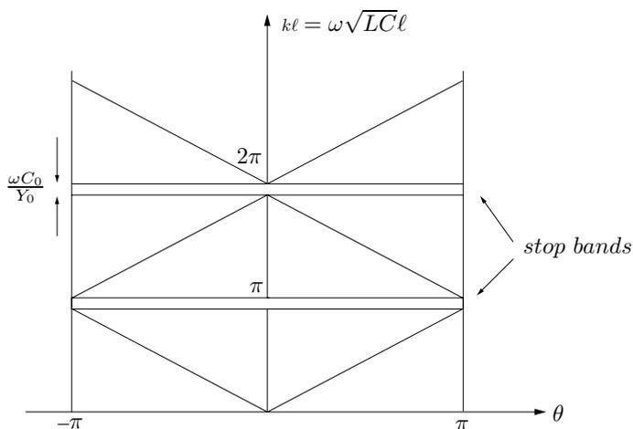
Figure E2.4.3.3 Bandpass lumped element line.
