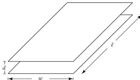
Figure 2.3.2 Parallel-plate transmission line with length  $\ell$ .
