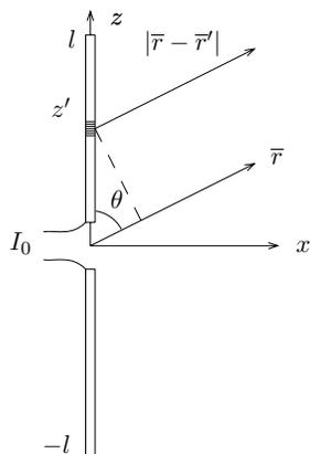
Figure 5.5.1 Wire antenna excited by a current source.
