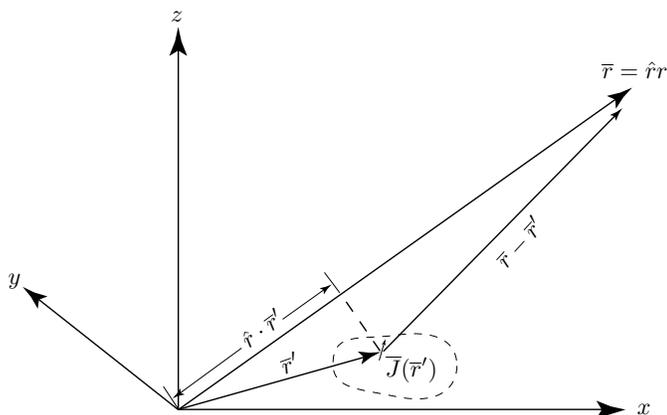
Figure 5.2.1 Observation point  $\bar{r}$  is outside the source region.
