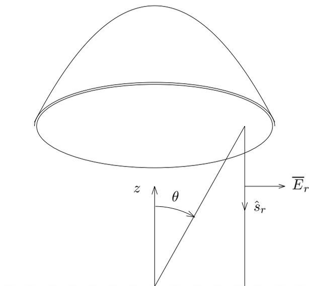
Figure 6.4.11 Paraboloidal reflector.
