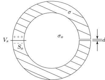
**Figure 2.1.7** Electric circuit excited by voltage source.
