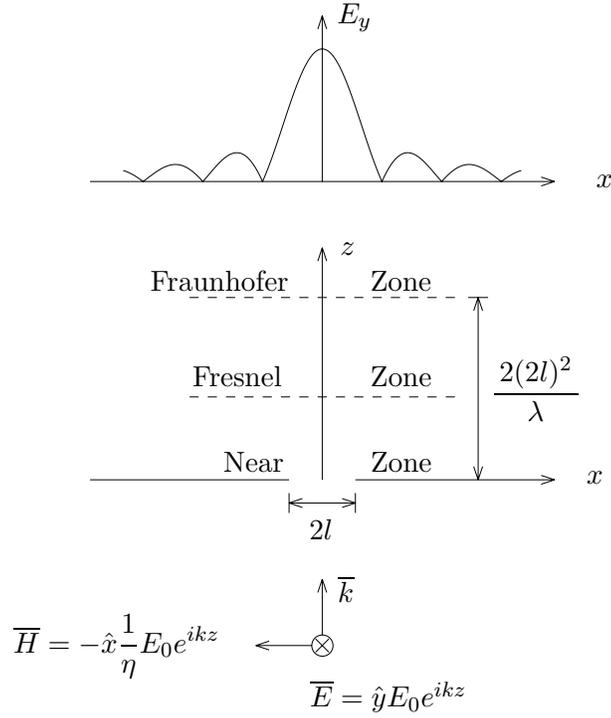
Figure 6.1D.1 Diffraction field in the Fraunhofer zone.
