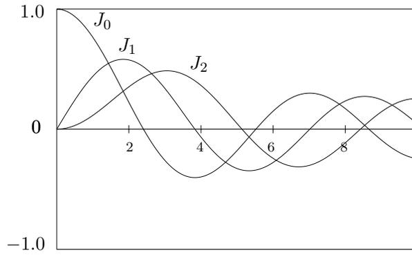
Figure 4.2.20 Bessel functions.
