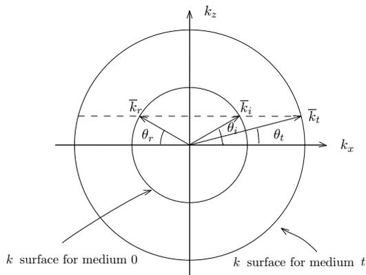
Figure 4.1.4 Phase matching using  $k$  surfaces.
