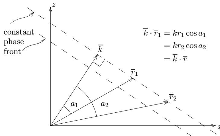
Figure 1.7.1 Constant phase fronts of a plane wave.
