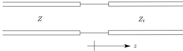
Figure 2.5.2 Transmission line modeling of reflection and transmission.
