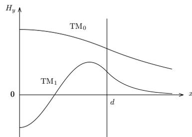
Figure 4.2.10 Magnetic field amplitudes for TM modes.
