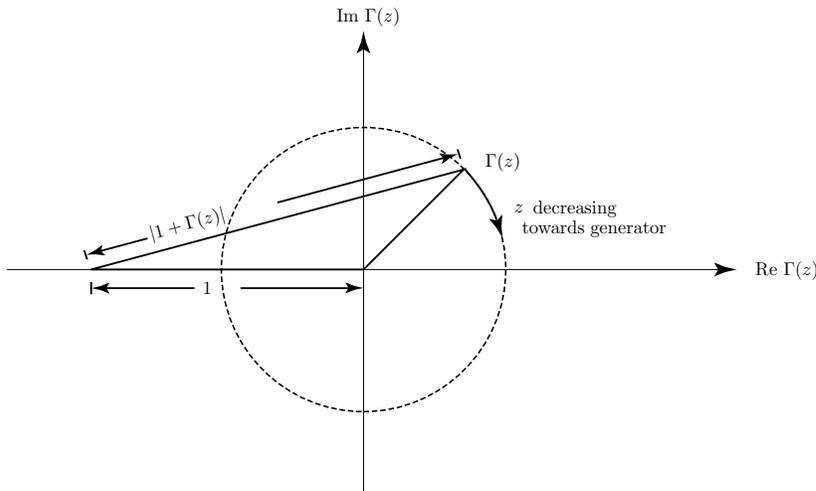
**Figure 2.3.5** Motion of  $\Gamma(z)$  on complex  $\Gamma$ -plane.
