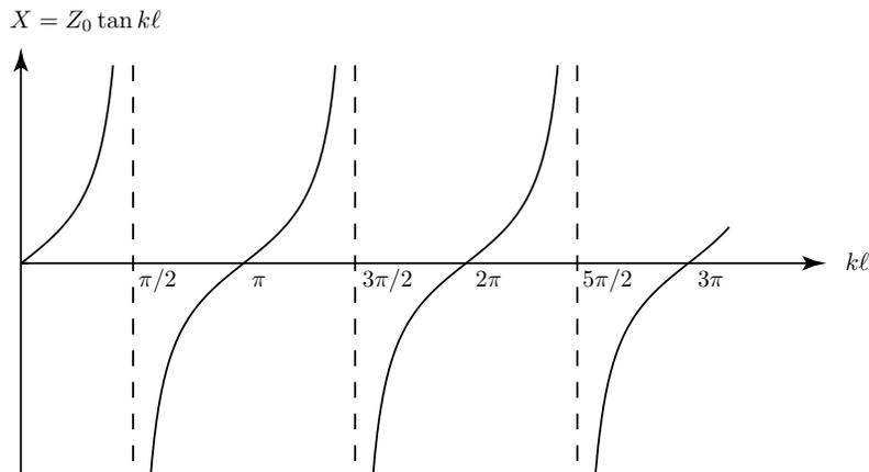
Figure 2.3.4 Reactance for short circuit transmission line.
