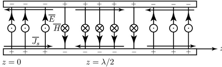
Figure 2.1.2 Surface charge and current on parallel-plate waveguide.
