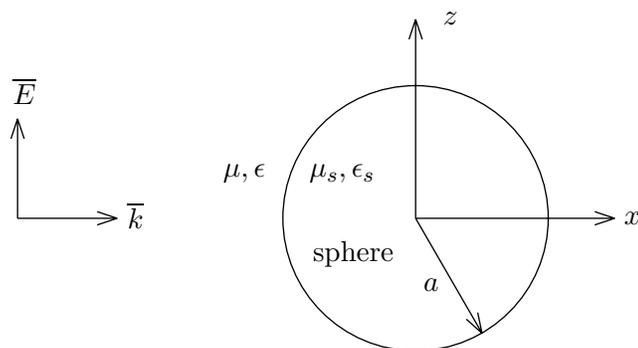
Figure 7.1.1 Rayleigh scattering by a small sphere.
