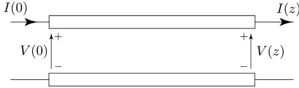
Figure 2.4.6 Two-port description of a transmission line.
