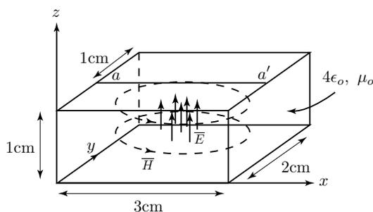
**Figure P4.3.1.1** Rectangular cavity.
