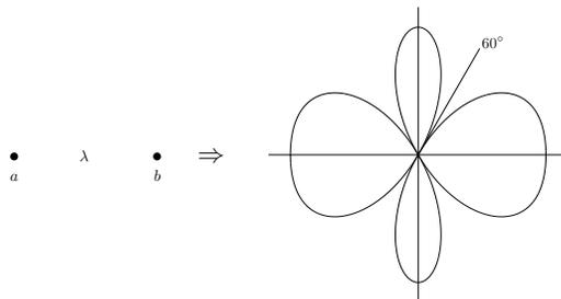
**Figure E2.5.3.3** Radiation pattern of two dipoles separated by  $\lambda$ .
