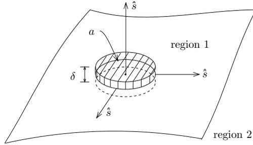
Figure 8.3.2 Pillbox for derivation of boundary conditions.
