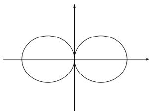
Figure 2.5.5 Radiation pattern for  $\lambda/2$  linear antenna.
