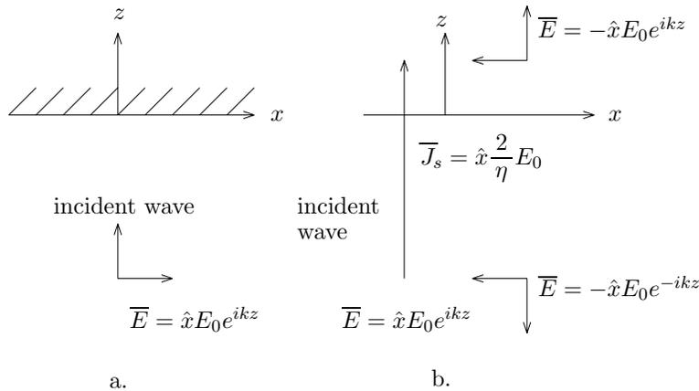
Figure E6.1.1.1 a. Plane wave incident upon a perfect electric conductor.
