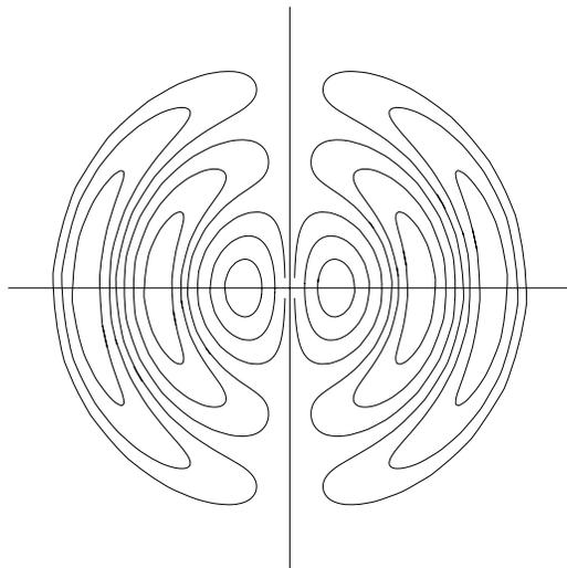
Figure 5.6.2 Electric field lines for  $\text{TM}_1$  mode.
