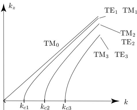
Figure 1.7.10  $\omega-k_z$  diagram.
