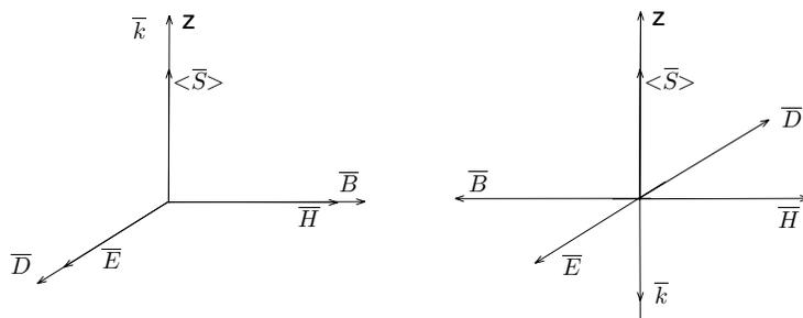
(a) Positive isotropic medium      (b) Negative isotropic medium
