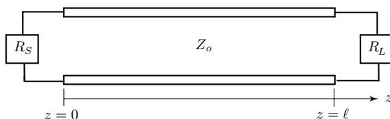
**Figure E2.2.6.1** Transmission line resonator.
