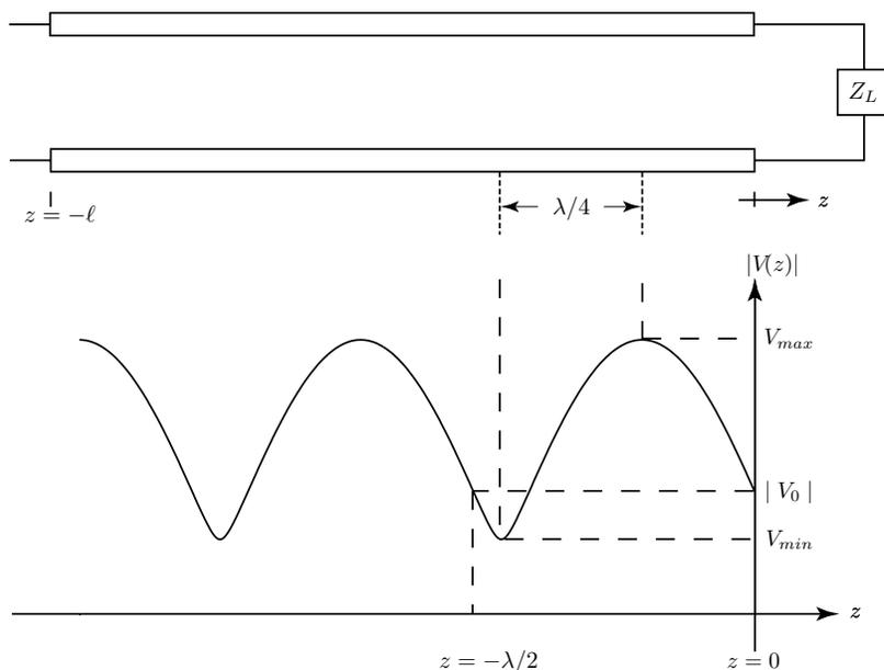
**Figure 2.3.6** Plot of voltage standing wave pattern.
