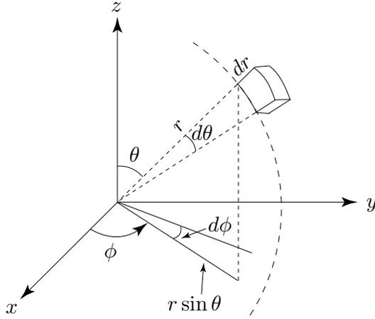
Figure 1.1.7 Spherical coordinate system.
