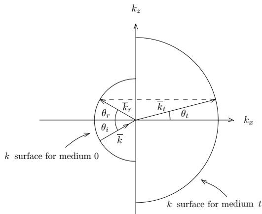
Figure 4.1.3 Phase matching using  $k$  surfaces.
