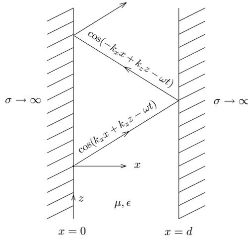
Figure 1.7.7 Parallel-plate waveguide.
