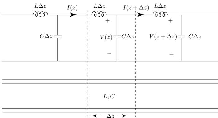
Figure 2.4.1 Lumped element approximation of transmission line.
