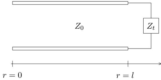
Figure 5.6.4 Transmission line model for the TEM mode.
