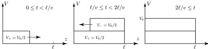
Figure 2.2.4 Transients on an open circuited line.
