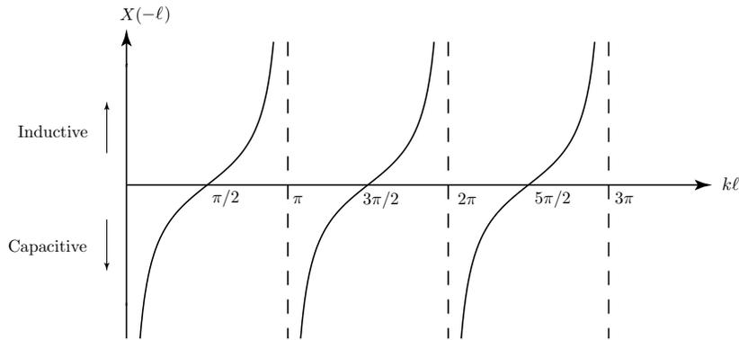
Figure 2.3.3 Reactance for open circuit transmission line.
