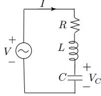
**Figure E2.3.3.1 Series R L C circuit.**
