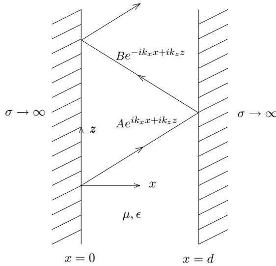
Figure 4.2.1 Parallel-plate waveguide.
