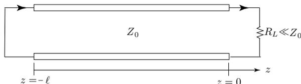
Figure 2.3.9 Transmission line resonator with small loss.
