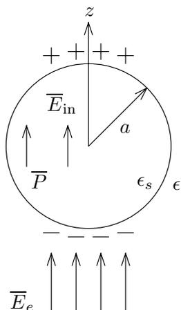
Figure 7.7.1 Sphere of radius  $a$  in a field  $\bar{E}_e$ .
