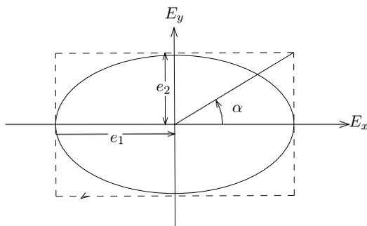
**Figure 1.2.9** Elliptical polarization.
