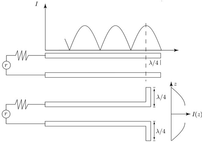
Figure 2.5.3 Current distribution on a half-wavelength dipole.
