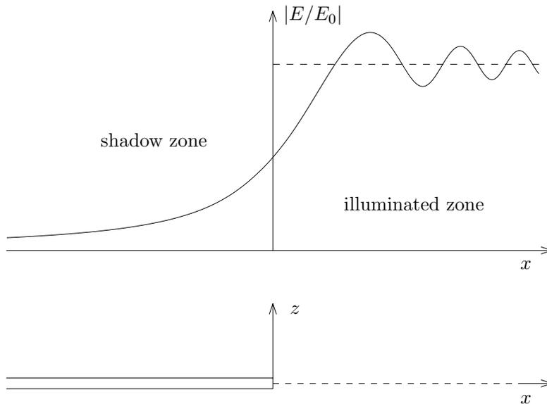
Figure 6.1D.4 Diffraction by a half-plane aperture.
