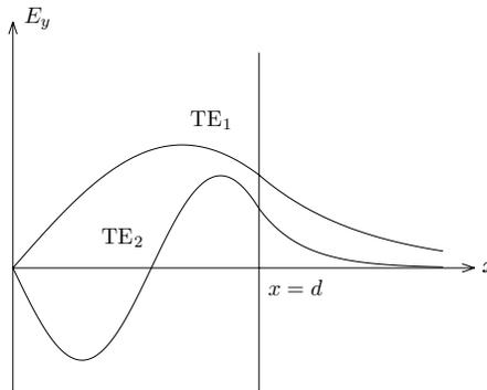
Figure E4.2.4.2 Electric field amplitudes for TE modes.
