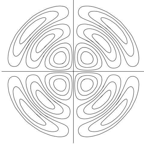
Figure 5.6.3 Electric field lines for  $TM_2$  mode.
