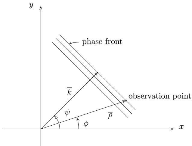
Figure 5.7.6 Cylindrical wave as superposition of plane waves.
